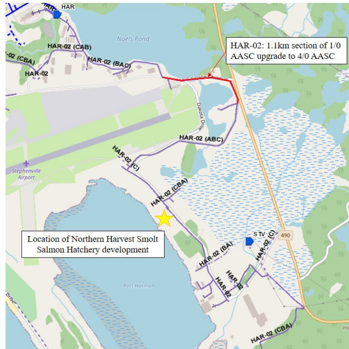
Figure 3: HAR-02 Distribution Feeder Upgrade
